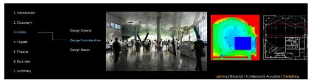
For daylight analysis, I typically use a Daysim analyze to show the solar gain distribution, with original floor plan on its side so audience can be more clear about what they are looking
